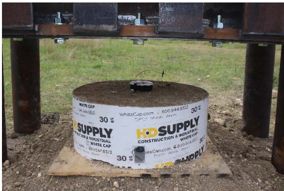
Test frame, specimen, and explosive pot
