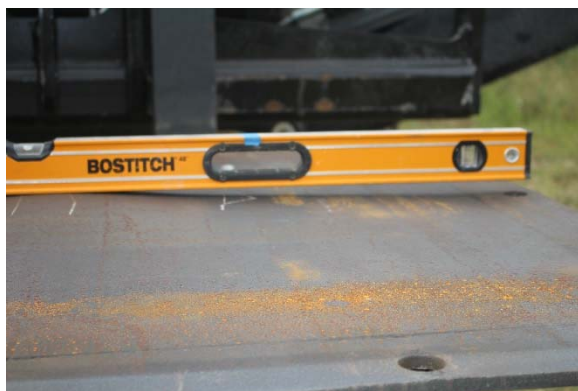
Post-blast permanent deflection, no breach
