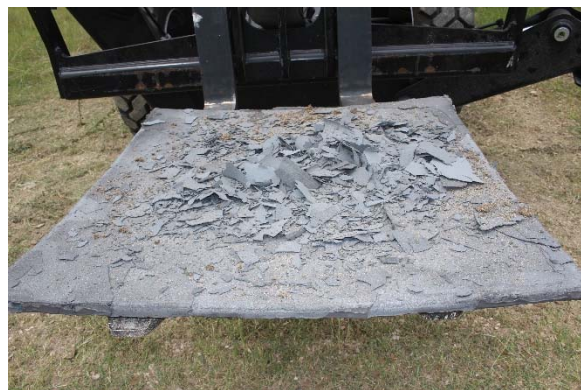
Ablative, energy absorbing layers, no breach
